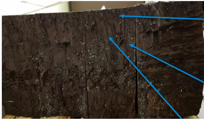
2. Columnar grains grow in the <100> direction from top of the slab
